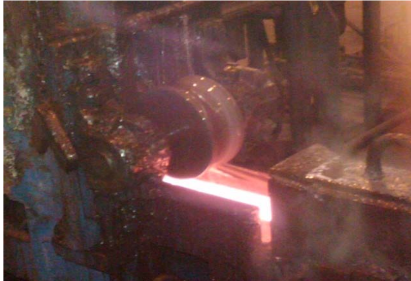
Figure 8. Roll from Carbide Composition at Hot (~ 950 °C) Rolling Manufacturing Facility.
